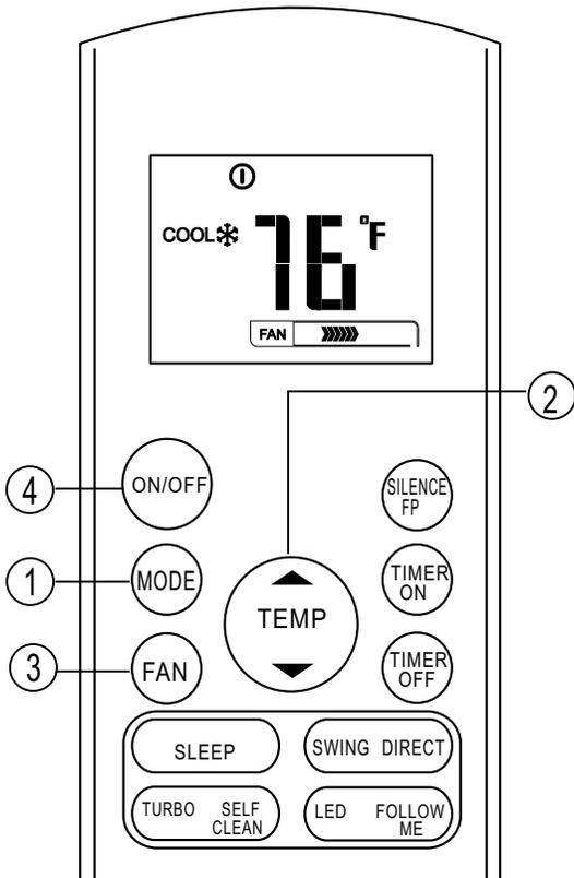
1. Press the **MODE** button to select COOL, HEAT (cooling & heating models only) or FAN mode.
